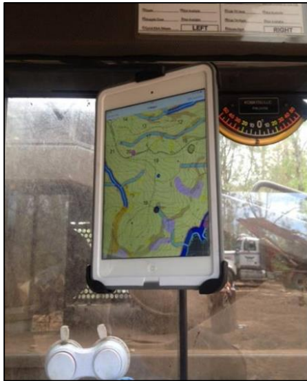
Figure 3: Example of the FCNSW developed Map Application in use in a harvesting machine showing its location in relation to mapped features such as harvest exclusion zones.
